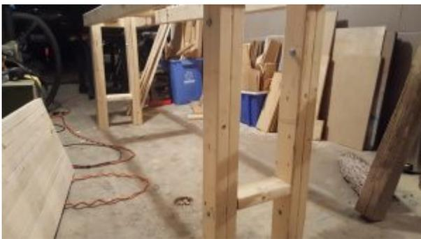
12. Now that the base is ready to go, your top should be as well. Next, place the top on the base and measure to insure it is even on all sides.
